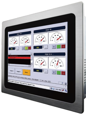
Real Flat Panel Mount (IP65 front side)
