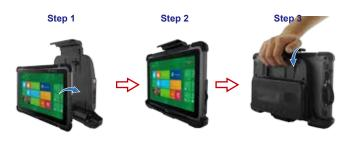
1 Insert the Tablet PC into the docking
