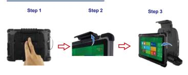
1.Slide the latch to open the hook
