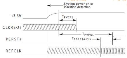
Note:  $T_{\mbox{PVCRL}}$  is measured from the later rising edge of +3.3V.
