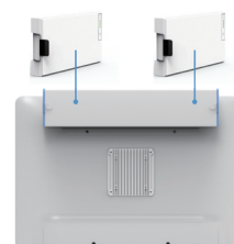
Battery module contains 2 x battery packs
