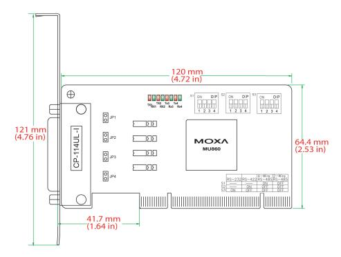
Onboard termination resistors can be activated individually for each serial port using jumpers JP1 through JP4. For CP-114UL, JP1/2/3/4 corresponds to serial port 1/2/3/4, respectively. For CP-114UL-I, JP1/2/3/4 corresponds to serial port 4/3/2/1, respectively. Short the jumper pins to activate the termination resistor; leave the jumper pins open to bypass the termination resistor.
